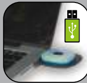
GREEN: BATTERY FULLY CHARGED
